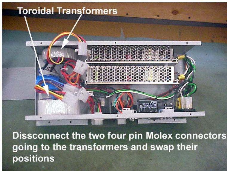
Both transformers plug directly into four pin Molex connectors, disconnect them and switch the connectors. The larger transformer goes to the four-pin connector with the orange jumper. The large transformer will now power the shooter motor and the smaller one will power the Halogen lamps.
