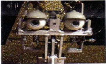
Step 8: On the back of the head-frame, there is the T-frame for the mouth cylinder. From the bottom of the top of the "T" measure down 3/4" and in the center of the frame mark for a hole, then 3/4" lower mark for another hole in the center of the frame.
