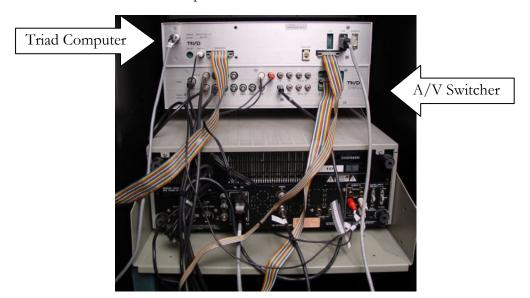
3. Now remove the top of the Triad Computer and locate the Cyperstar EPROM, as shown in the picture below.
