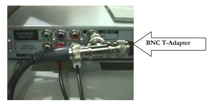
11. Connect one BNC to BNC cable from the T-Adapter and go to the Video In 1 input of the A/V Switcher.
