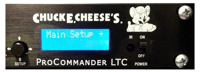
• Press the joystick to select Set IP Address.
