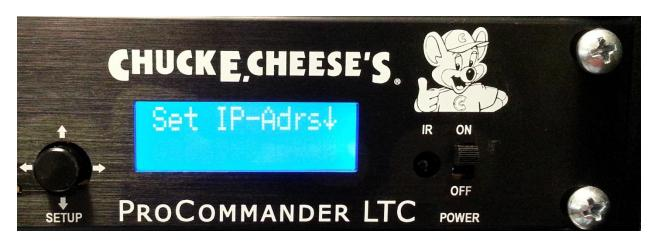
Using the joystick, set the IP Address to 010.000.000.101
