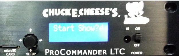
2. Move to the desired segment by using the joystick and then press in on the joystick to make the selection.
